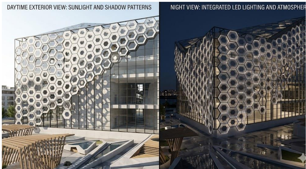
Figure 2. Photo-realistic visualization of a parametric façade system (case study: Youth Creativity Center)
