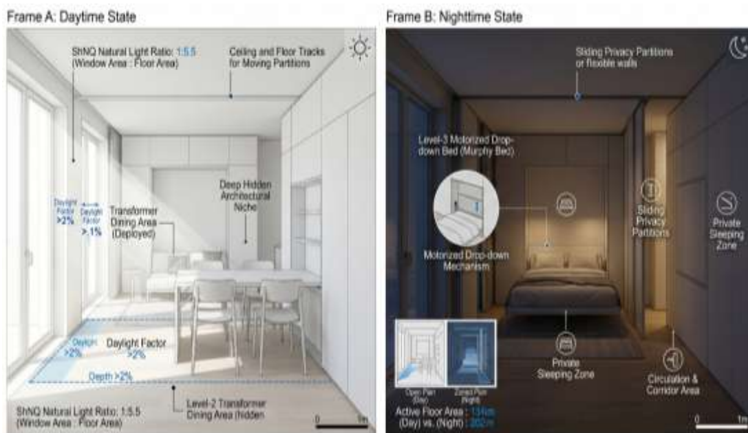
Figure 2. Implementation of Level-2 and Level-3 transformer systems in a 35 sqm flat
